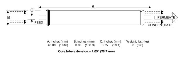
Notice: Permeate flow for individual elements may vary + or - 20 percent. All membrane elements are supplied with a brine seal, interconnector, and orings. Elements are vacuum-sealed in a polyethylene bag containing less than 1.0% sodium meta-bisulfite solution, and then packaged in a cardboard box.
