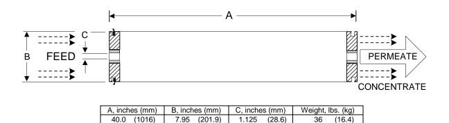
Notice: Permeate flow for individual elements may vary + or - 15 percent. All membrane elements are supplied with a brine seal, interconnector, and o-rings. Elements are vacuum sealed in a polyethylene bag containing less than 1.0% sodium meta-bisulfite solution, and then packaged in a cardboard box.
